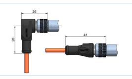
For sensors with connector output the cable has to be ordered separately. You can choose from a cable with a straight connector or with an angular connector.
