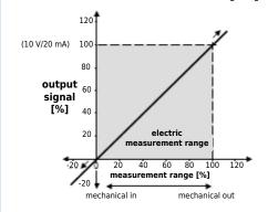
The output signal is referring to the electric measuring range. If the sensor is operated outside the measuring range or the measuring range is exceeded, the signal is also outside the defined range (i.e. > 10V/20 mA or < 0 V/4 mA, in the graph: > 100 % or < 0 %). Please keep this in mind for control systems with cable break detection lower than 4 mA or for a maximum input voltage > 10 V of measuring instruments. If necessary install the sensor **before** connecting to the PLC.
