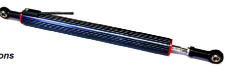
The SM19 series of linear potentiometers are designed to withstand the harsh environments of testing and industrial applications. Using proven 'Conductive Plastic' technology, the sensors offer high performance and reliability at operational temperatures up to +150°C
